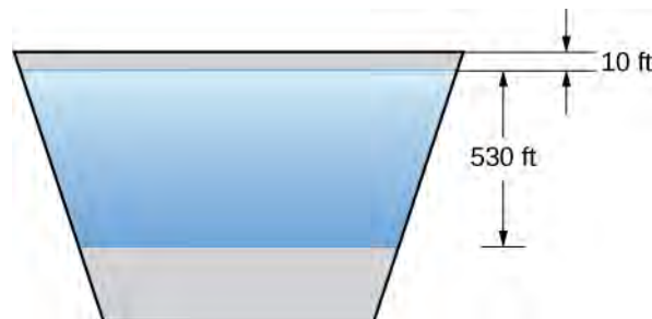
Figure 6.59 A simplified model of the Hoover Dam with assumed dimensions.
